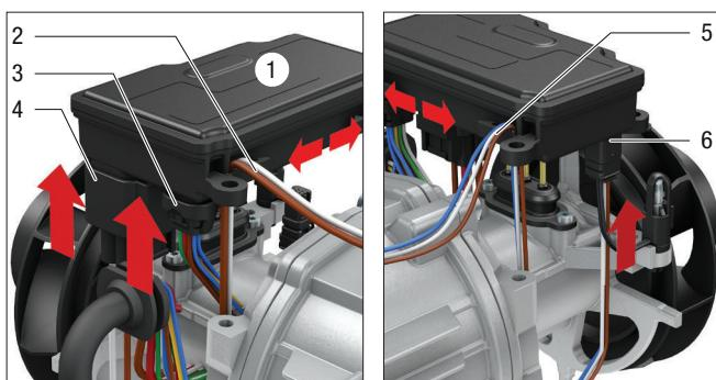
1 Control box 5 Combination sensor lead harness
