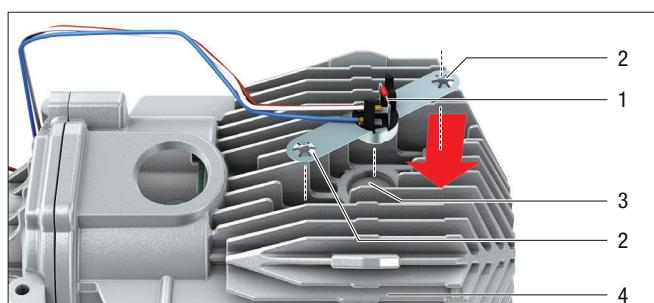
1 Combination sensor    3 Retaining recess
