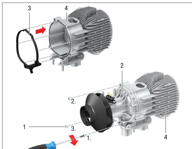
1 Fixing screws M5 × 20 (Torx)    2 Fan
