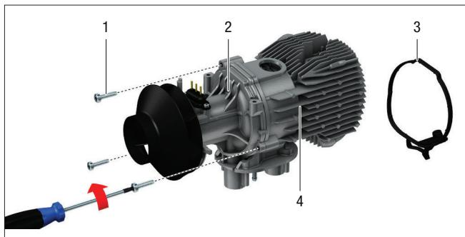
1 Fixing screws M5 x 20 (Torx)    2 Fan
