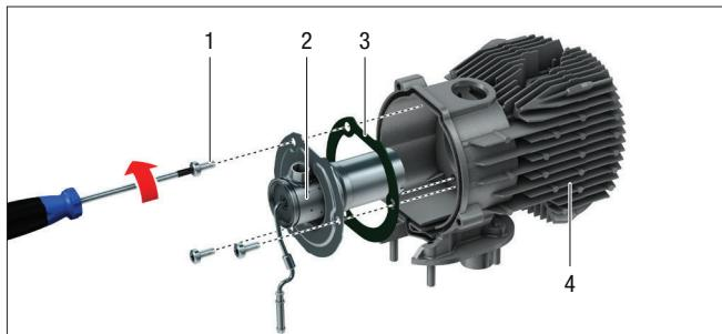
1 Fixing screws M5 x 12 (Torx)
