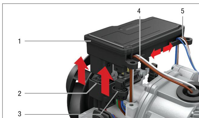
1 Control box      3 Connector, cable harness
