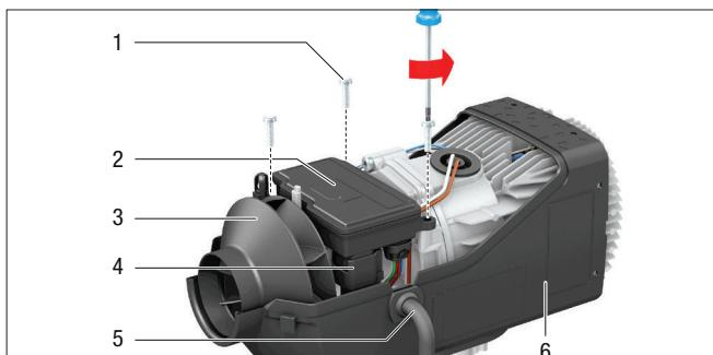
1 Fixing screws M4 x 16 (Torx) 4 Connector, control box
