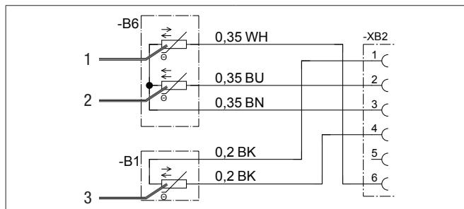
1 NTC overheating sensor 50 kΩ      3 Air inlet sensor
