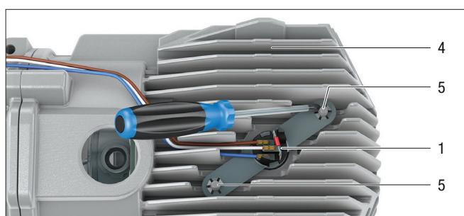
1 Combination sensor    3 Retaining recess
