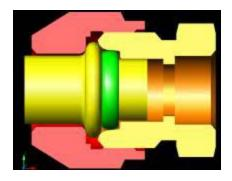
The o-ring must be compressed to ensure a good seal.
