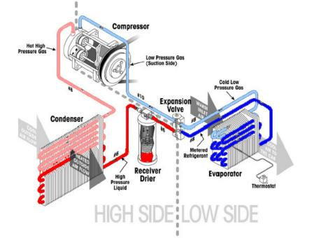
The air conditioning system is divided into two sides, the high side and the low side. This illustrates the flow of refrigerant through the system.
