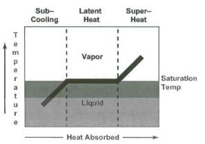
Latent heat is the heat required to make a liquid at a certain pressure turn into a vapor at that pressure. The saturation temperature changes with the pressure of the refrigerant.
