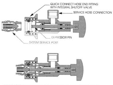
VALVE ASSEMBLED TO SERVICE PORT WITH VALVE IN THE OPEN POSITION
