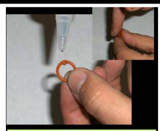
Drip clean oil onto clean o-ring. Smooth onto entire surface.
