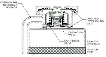
The pressure radiator cap seals the cooling system at the inlet on top of the radiator. Caps are pressure rated to match cooling system design. Each pound of pressure on the cooling system raises the boiling point of coolant three degrees Fahrenheit, so the pressure cap extends the cooling system operating range above the normal boiling point. The cap pressure valve opens when operating pressures are high. Coolant can flow through the heater core regardless of thermostat position.
