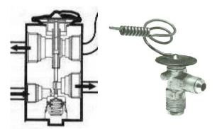
The expansion valve restricts the flow of refrigerant, to provide the pressure differential the system needs for the refrigerant's temperature and boiling point to increase and decrease.
