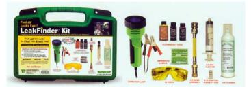
One way to make your leak-finding chores easier is with a black light. You inject a small amount of dye into the air conditioning system, and run the black light along the system lines and fittings. Any leaks in the system will show up a luminous green.
