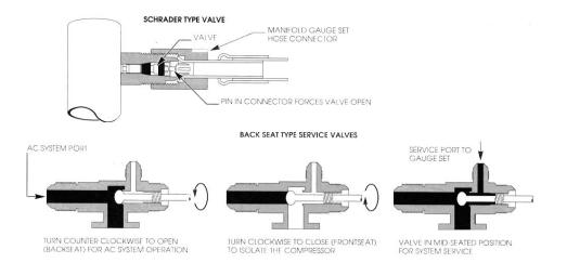
The valve drawings are cutaway. The Schrader valve in the upper portion of the illustration (like a tire air valve) is either closed or open. The three illustrations above show and describe stem type valve operations.
