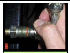
Align fittings and ensure seal is seated correctly.
