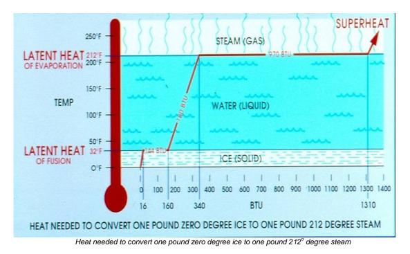
The point to remember here is even though you added 970 BTUs to the water, the water temperature never went over 212°F (100°C). That 970 BTUs was the energy necessary to change the state of the water from a liquid to a gas (vapor). The extra heat being absorbed is known as *"The Latent Heat of Evaporation,"* or Latent Heat.
