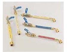
Whether you're using gauges or a recycling machine to service or diagnose a system, you must have shutoff valves no more than 12" from the ends of the hoses.
