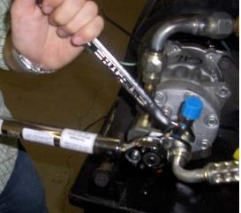
Tighten connection with proper torque. Use a backer wrench to avoid twisting parts.
