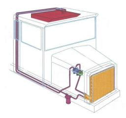
Make sure the service ports all have caps screwed on. These caps are the primary seal for service ports. If any caps are missing, you must replace them as part of the service. Those caps are more than dust covers – they help prevent refrigerant from escaping into the atmosphere.
