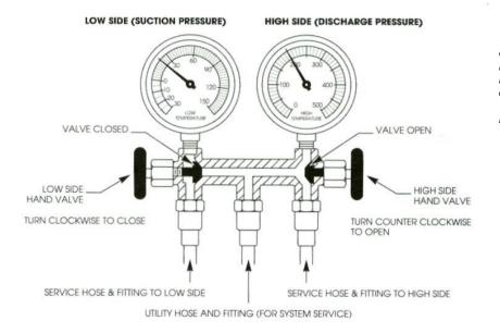
The figure below illustrates a basic manifold gauge set and explains how it works.
